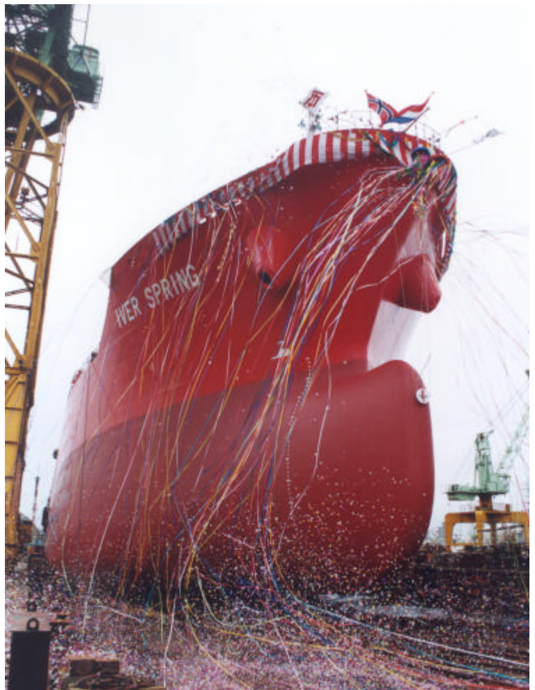
A 25,000 dwt Chemical Tanker being launched in Japan
