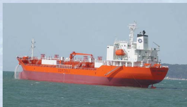
M. T. Bow Asia and M. T. Bow Singapore - 9,900 MT DWT Type II/III Chemical tankers delivered from Fukuoka Ship yard in 2004.
