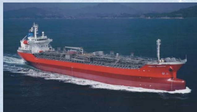
M. T. Chemical Marketer - 14,000 MT DWT, Type II/III Chemical tanker, delivered 2004 from Asakawa Shipyard.
